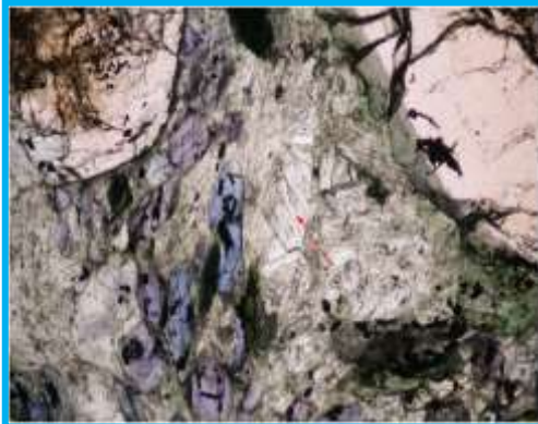
c. high relief of garnet, fibrous of talc crystals with relics of amphibole slightly to completely altered to chlorite. PPL, X150
